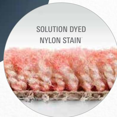
\*Results of stain test using solution-dyed nylon 6 carpet
